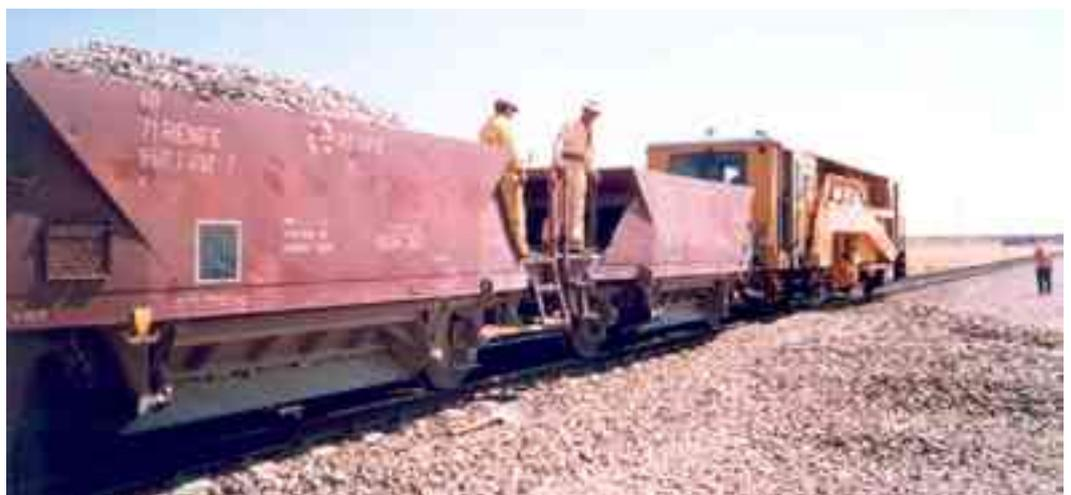
These Works for the Spanish National Rail Network (Renfe) consisted of replacing eleven C-type diversions and eliminating the corresponding dilation apparatus, installing points heaters and renovating the electro-hydraulic switches. This work was done at El Campillo, Cantalpino, El Pedroso de la Armuña and Gomecello stations, also renewing the sleepers with MR-93 concrete single-block units.
