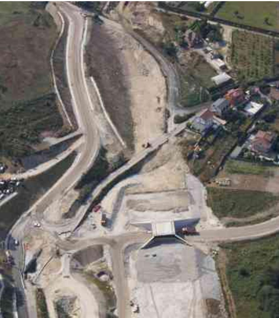
Within the range of the works a viaduct at Pexegueiro shall be built, made up of a hyperstatic slab of lightweight prestressed reinforced concrete with spans of 20+25+25+20 m, having used set in making the slab, possible due to the low height of the piles.
