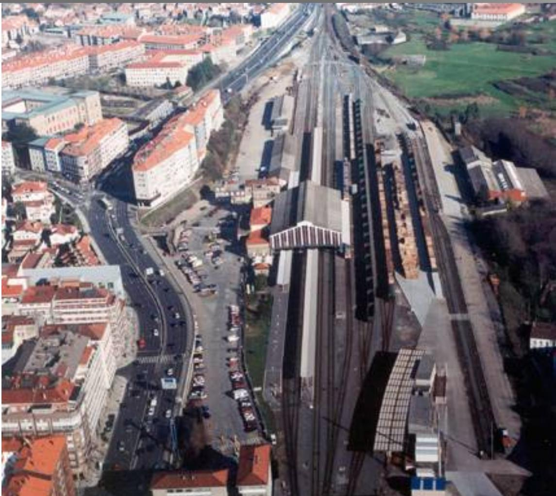
These works, developed by the Ministry of Development through the Railways Department, is divided into two clearly differentiated parts: the renovation and remodelling of the fan of tracks at the northern head of Santiago station, and the doubling and renovation of the track along the first seven kilometres of the Santiago – La Coruña section.
