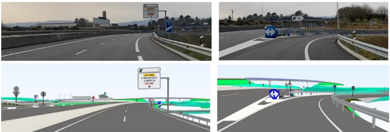
Figure 2 - Comparison between images taken "in situ" and images extracted from a 3D road model
